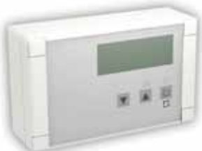
CT – Total Control Suitable for all models from Optima to Max (except Minibel). Auxiliary devices: anti-freeze sensor, door contact, thermostat, etc... Time programmer: 3 ON/OFF for each different day of the week. Digital display with hour, fan speed, heating stage, temperature... Multilanguage display 9 languages. Manual or automatic functioning with programmable behaviours.
